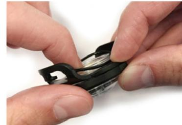
7. Place the o-ring back in its groove.
