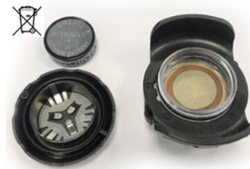
3. Remove the old battery pack and dispose of it correctly.
