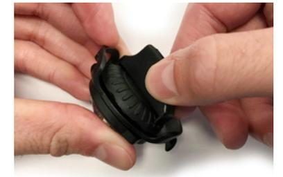
8. Use the Service Tool to screw the light back together.
