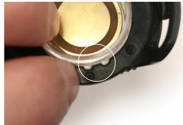
6. Place the mount back on top of the guide pins.<sup>2</sup>
